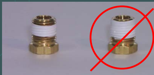
Use Teflon Tape Correctly
